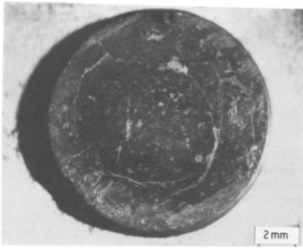
Figure 3 Sectional view of the polished front surface of \text{Si}_3\text{N}_4 compacted at 64 GPa.
