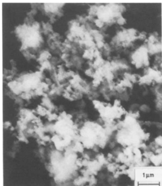
Figure 1 Scanning electron micrograph of \text{Si}_3\text{N}_4 starting powder.
